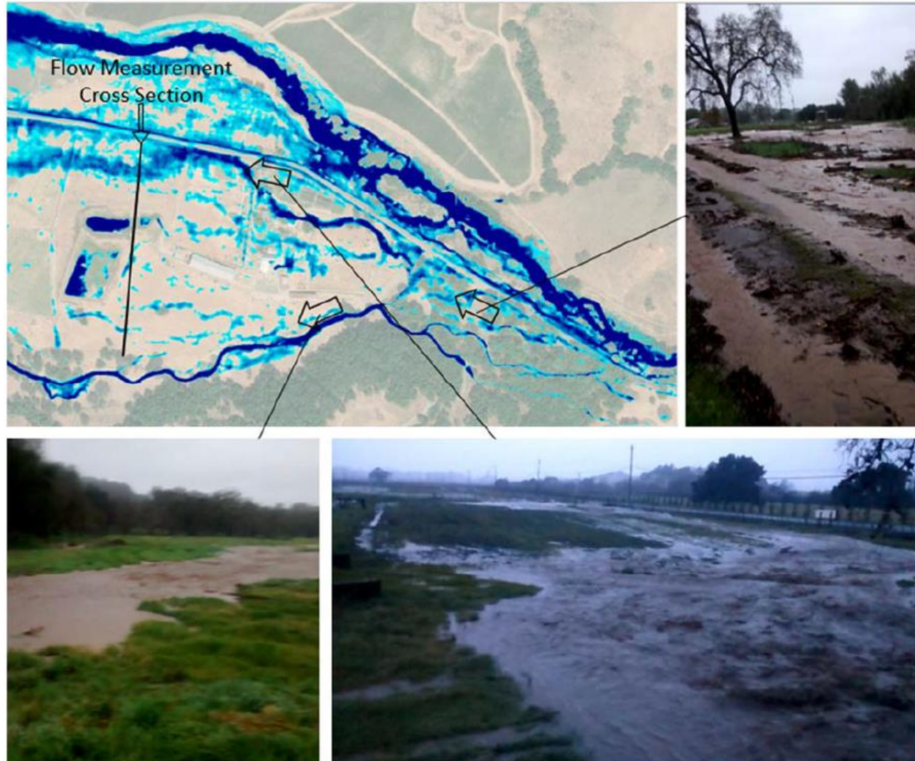
Figure 8. Existing condition hydraulic model results compared to photos taken during the Jan 8 th , 2017 flood. (Photos taken by the landowner Alex Perotti)
